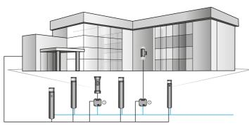
① The DALI actuator (item no. EP10427473/ EP10427480) switches on the "master" light if movement is detected in the field of detection
